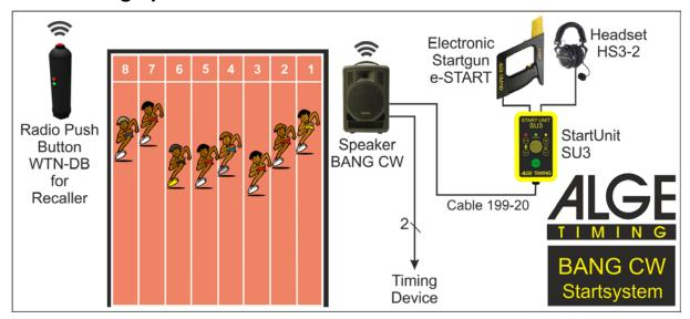
The BANG CW is suitable for indoor use only. Protect it against dripping water and splash water, high air humidity, and heat (admissible ambient temperature range 0 - 40 °C).
