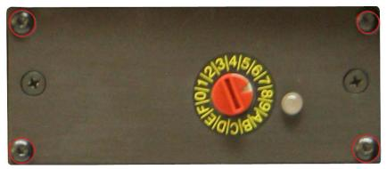
When the screws are removed, you can pull out the unit.
