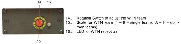
The **ALGE** Wireless Timing Network WTN is a compact radio system for timing and is equipped with the most updated technology. The BANG W has a WTN-radio module built in and is fully compatible with the WTN
