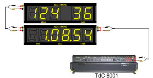
For the *A*LGE TDC4000 use cable 010-01. As soon as the display of the *A*LGE TDC4000 shows a running time, the GAZ should also show it (otherwise twist the connection plug at *A*LGE TDC4000 by 180° degrees).
