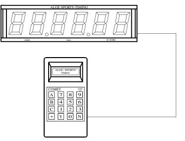
Cable 030-10 is a 3-wire cable, which supplies the ALGE Comet from the display board.
