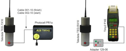
With the adapter 129-06 it can be set if it is a start or stop impulse. This is of advantage if only one photocell is used for a circuit.
