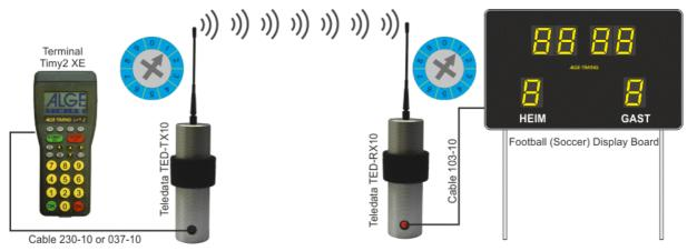
In order to supply the TED-TX by the Timy, cable 108-10 is required. It is recommende to supply the Timy by an *A*LGE power supply unit.
