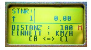
If the start-photocell is triggered out, the display will show instead of "0.00" a dotted line. Timy will calculate from the adjusted distance and min. speed, how long one cycle will take at maximum. If this time will be crossed, the display will show "0.00" and is ready for the next measurement.
