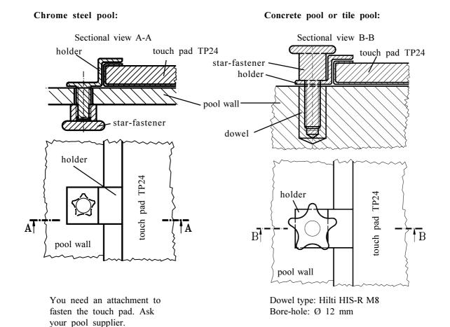
If your use the touch pad TP24 in a swimming pool with a lane width of 2.5 m it is possible to fix two touch pad with one holder and one star-fastener.
