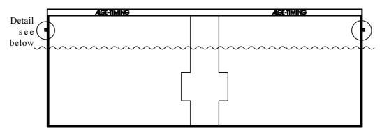
The touch pad holder of the touch pad has a M6 screw, which is fixed on both sides just above the water level. You have to attach the touch pad to the pool wall that it is 30 cm above the water and 60 cm below the water.
